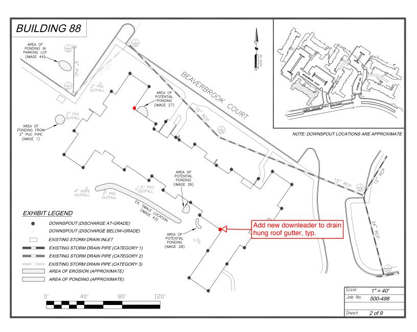
Additional downleader locations noted on the plans assume resloping of gutters at their midpoint to drain half the gutter to the new downleader and half to the existing.
